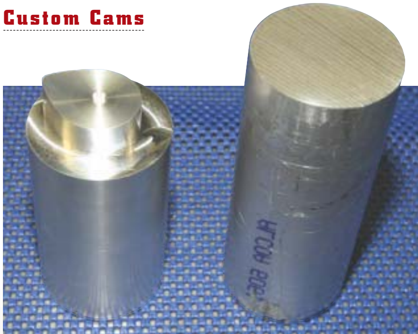
On the left is the finished pattern, which is a life-size replica of the actual lobe. On the right is the raw material from which the pattern is cut.
